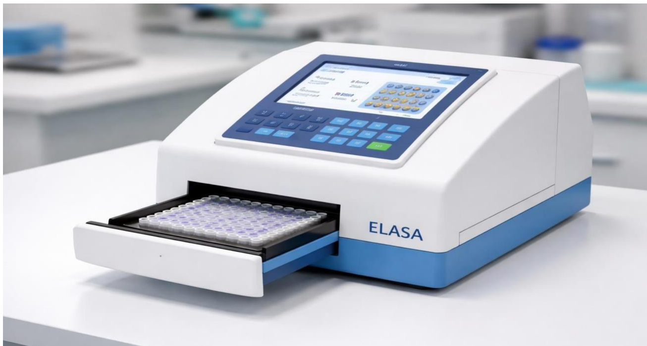
Figure (1): ELISA Reader used for measuring the concentration of antibodies or hormones in biological samples through colorimetric changes within the microplate wells.
