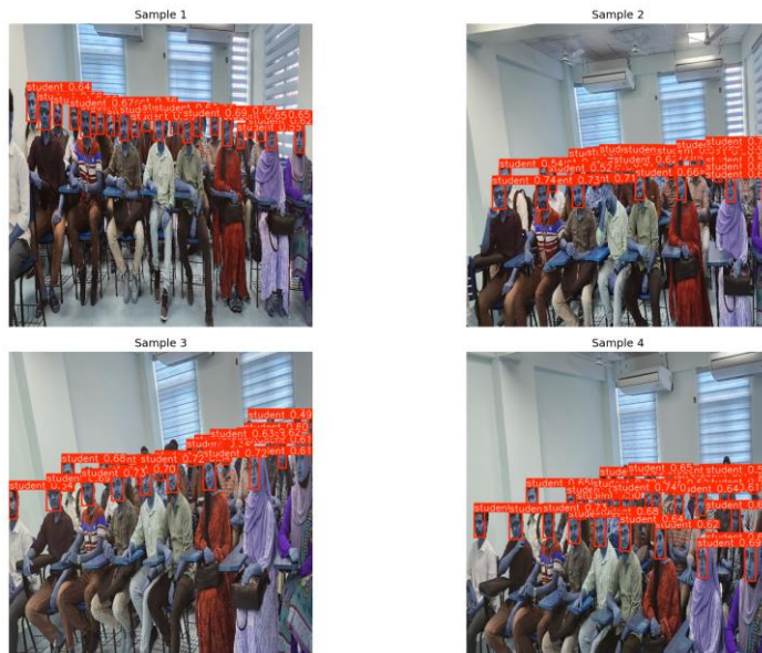
Fig. 5: Student-YOLOv8 detections on unseen classroom images with confidence scores.
