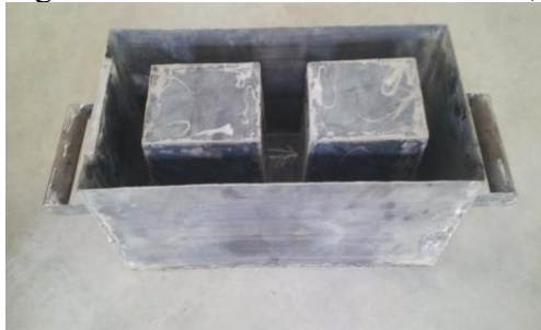
Figure 3.1: 225mm×225mm×450mm, with hollow sizes 187.5 mm×175 mm mould
