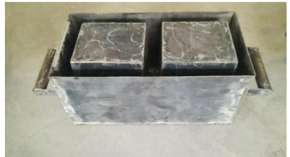
Figure3.3: 225mm×225mm×450mm hollow size with hollow sizes 173 mm×190 mm
