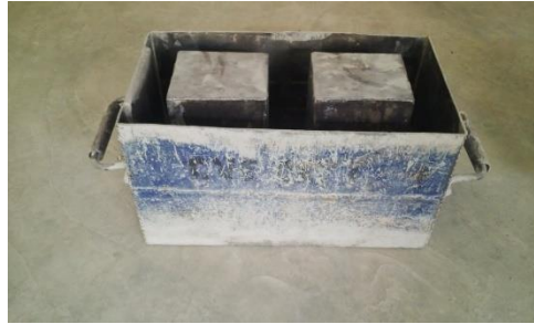
Figure 3.1: 225mm×225mm×450mm, with hollow sizes 187.5 mm×175 mm mould
