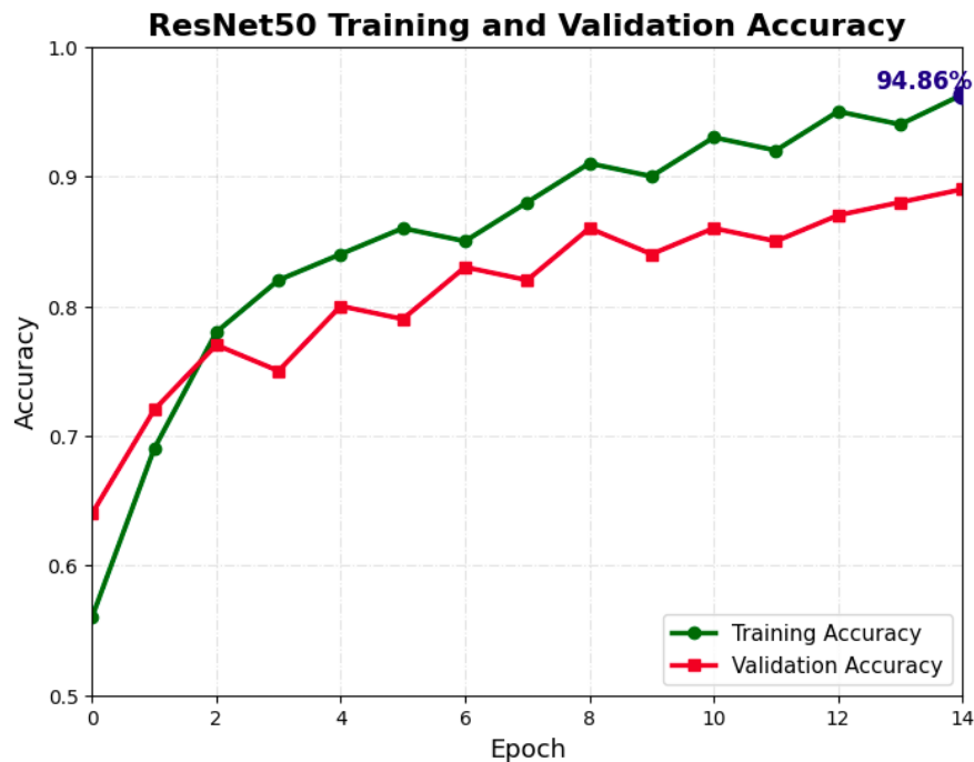
Figure 4.1: Training and validation accuracy curves of the proposed ResNet50-based CNN
